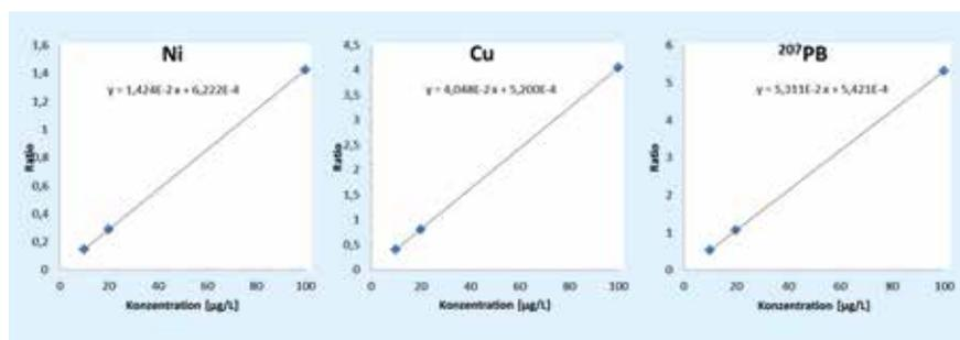
3 Calibration curves of nickel, copper and 207Pb. The y-axis shows the concentration of the respective element in  $\mu\text{g/L}$ . The x-axis depicts the ratio of the signals of the respective element to rhenium used as the internal standard (10  $\mu\text{g/L}$ ).
