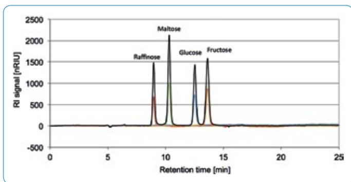
Fig. 2: Separation of individually injected sugar samples and of a sugar mixture using a RNM Carbohydrate Na<sup>+</sup> 8% column with ultrapure water. Black curve: sugar mixture
