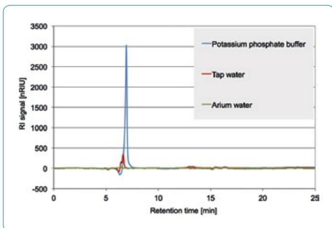
Fig. 3: Chromatograms of 2 µl of 10 mM of potassium phosphate buffer, 2 µl of tap water and 2 µl of Arium ultrapure water
