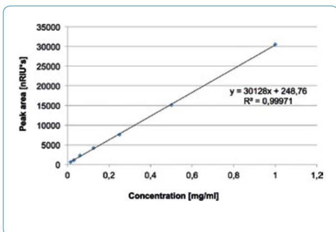
Fig. 4: Standard series for raffinose (values from Table 2) passed through a Rezex RNM Carbohydrate Na<sup>+</sup> 8% column with Arium pro VF ultrapure water
