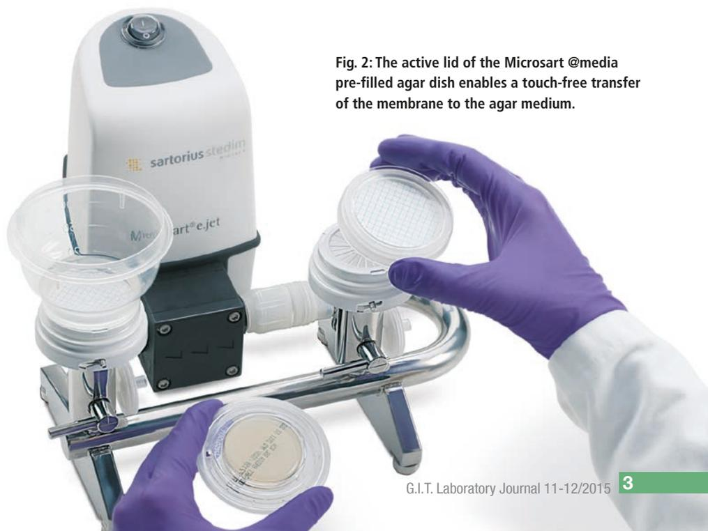
**Fig. 2:** The active lid of the Microsart @media pre-filled agar dish enables a touch-free transfer of the membrane to the agar medium.
